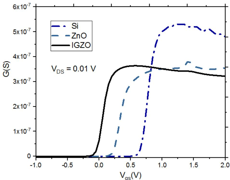
**Fig. 6:** Transconductance versus gate voltage. The silicon device has higher maximum transconductance and performs better due to lesser fixed charge
