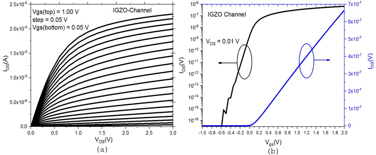
**Fig. 3:** (a)  $I_{DS}/V_{DS}$  for varying  $V_{gs}$  from 0.05 V to 1.00 V with steps of 0.05V (b)  $I_{DS}/V_{gs}$  Linear characteristics Subthreshold characteristics of Simulated IGZO FinFET structure
