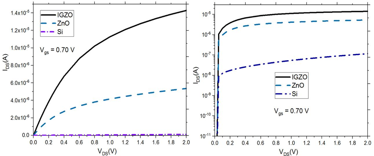
**Fig. 5:** A plot of drain current versus drain voltage comparing IGZO FinFET with the Si FinFET and ZnO FinFET. The graphs depict (a) in the linear region (b) in the subthreshold region
