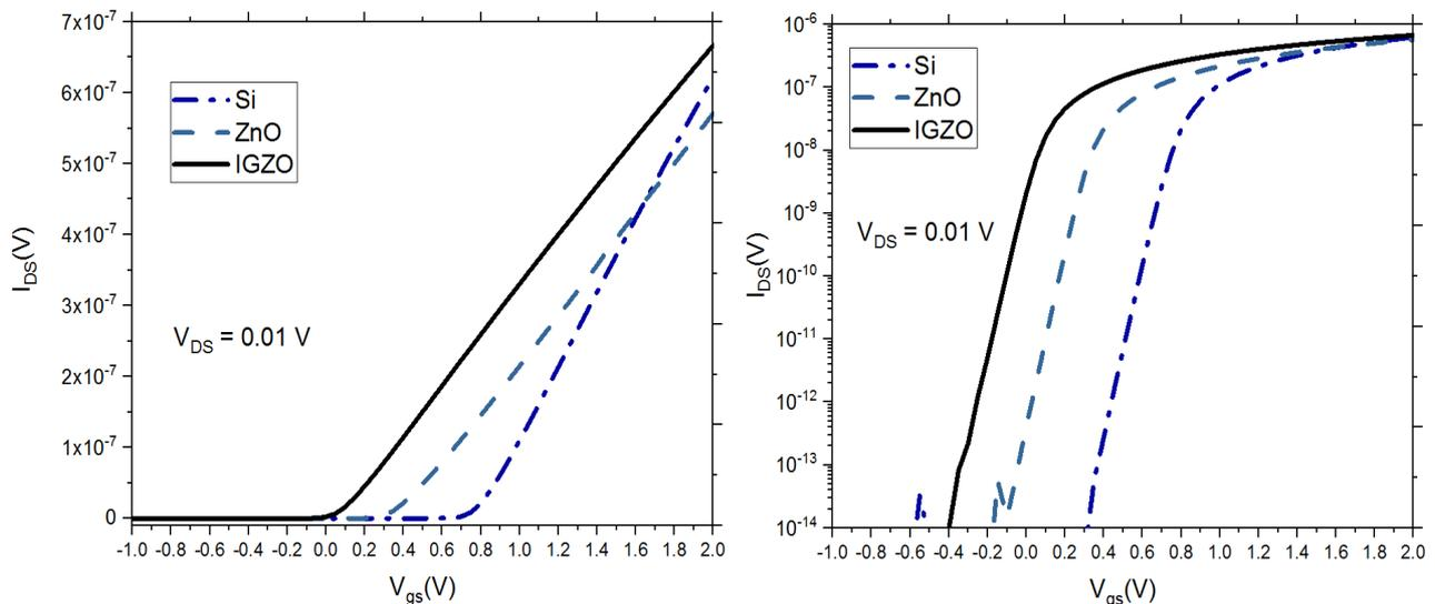
**Fig. 4:** A plot of drain current versus gate voltage comparing IGZO FinFET with the Si FinFET and ZnO FinFET. The graphs depict (a) in the linear region (b) in the subthreshold region
