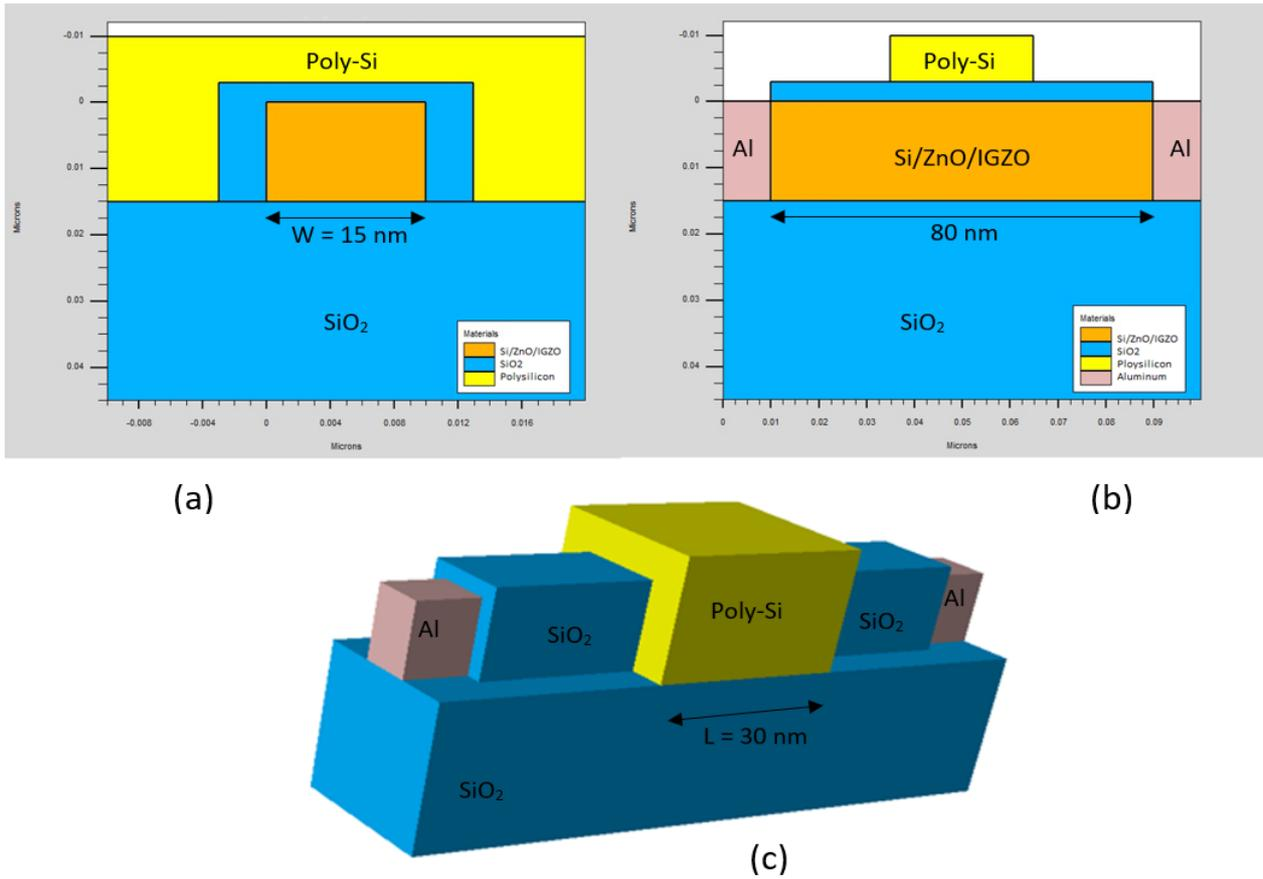
**Fig. 1:** Simulated devices having various material channels (Si, ZnO and IGZO) (a) 1-D plane showing the width of devices (b) 1-D plane showing the length of devices (c) 3-D plane showing devices
